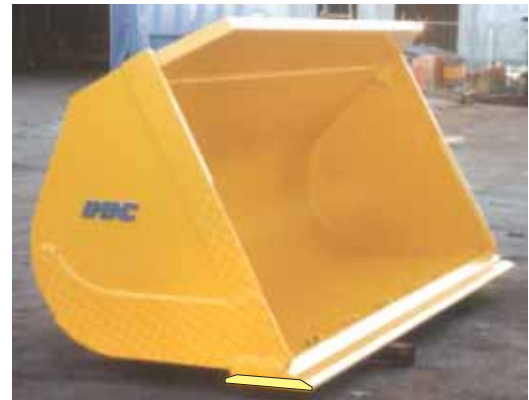
Bolt-on Cutting Edge & Outside Wear Plates with Hard Facing
