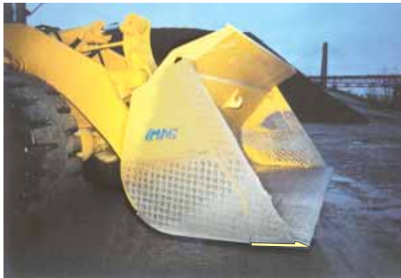
Weld-on Half Arrow Edge & Extra Large Wear Plates with Hard Facing Inside and Out
