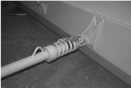
PUSH POLE Spring Cushioned - Telescopic c/w Shear Pin
