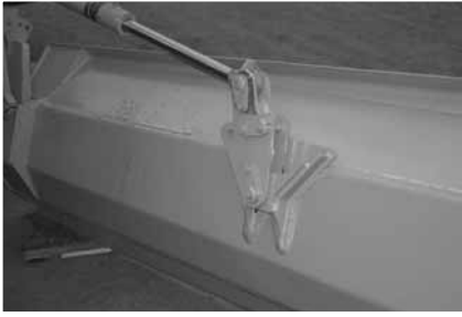
OUTBOARD FLOAT MECHANISM with Override Capability for Positive Downpressure
