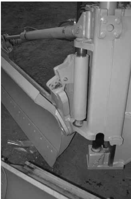
INBOARD FLOAT with Override Capability for Positive Downpressure & PITCH CONTROL with Shear Pin
